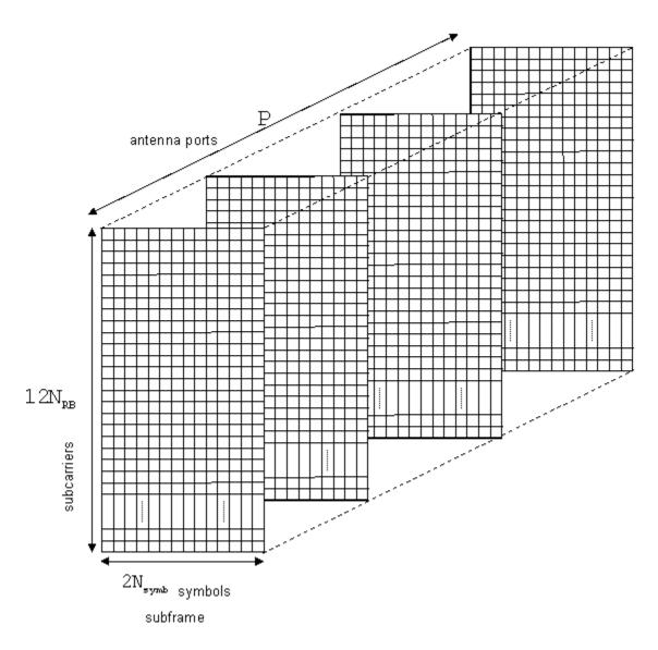
The rows of this array represent the subcarrier. The columns map the OFDM or SC-FDMA symbols in the downlink and uplink, respectively. The third dimension or plane represents the antenna ports. In the LTE System Toolbox, the resource grid spans a subframe in the time-domain, instead of a slot. Hence, the documentation uses the term subframe
