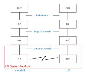
LTE System Toolbox focuses on the physical layer, which is highlighted in red in the preceding figure. It also supports interfacing with portions of the RLC and MAC layers, which are highlighted in blue. The primary features of the LTE physical layer are OFDM modulation, including the time-frequency structure of the resource blocks, adaptive modulation and coding, hybrid-ARQ, and MIMO.
